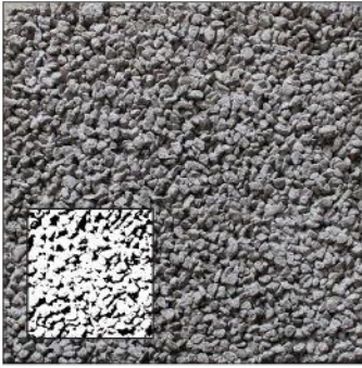
TEST PANEL 1 -target void ratio 25% -1" crushed stone -w/c ratio = .6
