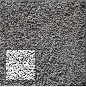
TEST PANEL 3 -same mix as panel 2 but with exposed aggregate
