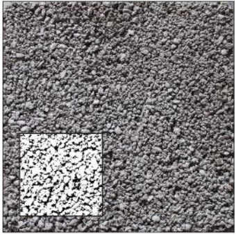
TEST PANEL 2 -1" crushed stone 76% -sand 24% -w/c ratio = .6
