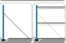
The roof and floor is connected to the walls and bracing is removed
